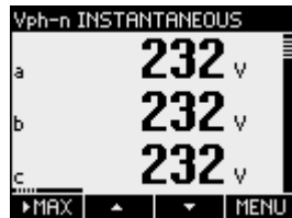
Figure 3-1 Display of the measured voltage in the case of connection type 3P4W
