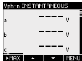
Figure 3-2 Display of the measuring voltage in the case of connection type 3P3W
